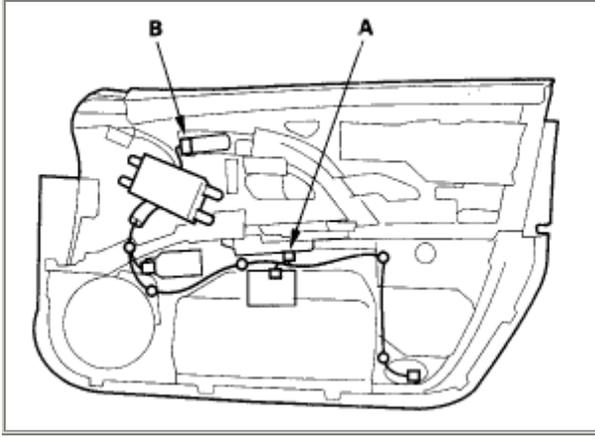
8. Disconnect the power window switch connector (A) and the seat position memory switch connector (B).
