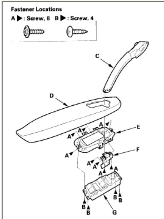
10. Remove the screws (A, B), then separate the door grip (C), the armrest (D), the power window switch panel (E), the grip bracket (F), and the power window switch (G).
