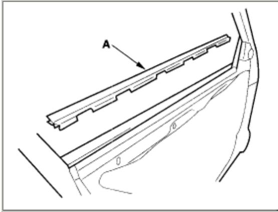
6. If necessary, remove the door glass inner [weatherstrip](#) (A) from the door by pulling it up.
