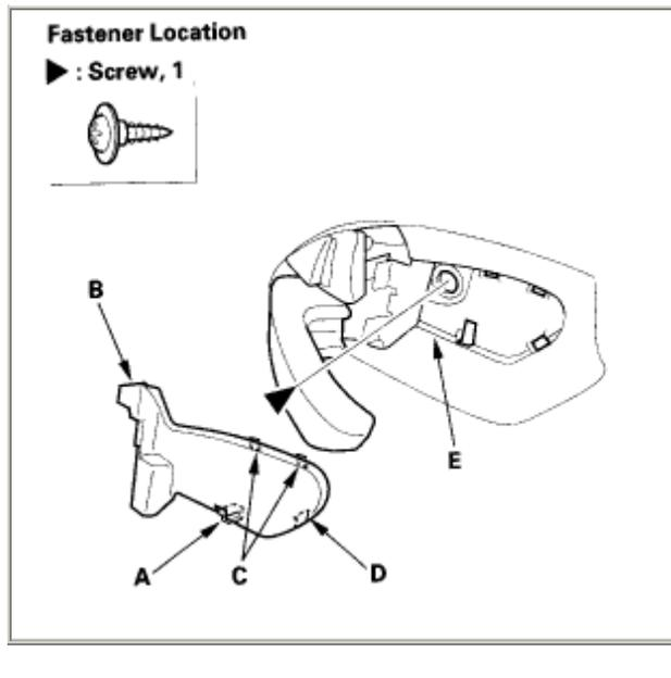
1. Using a trim tool, push on the bottom hook (A) and pivot the cover (B) on the upper hooks (C), then detach the front hook (D), and then remove the cover and the screw securing the inner handle (E).
