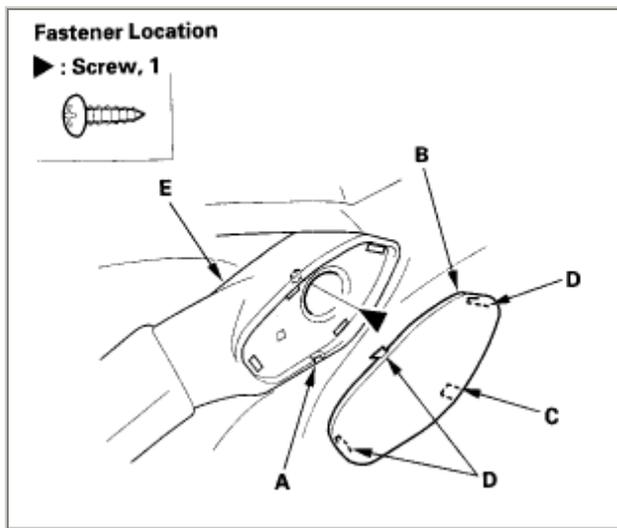
3. Using a trim tool, pry out the notch (A) of the grip cover (B) to detach the hook (C), and then pull out the cover to release the remaining hooks (D), then remove the cover from the grip (E).
