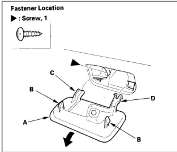
2. Using a trim tool, pull the top edge of the pocket light cover (A) out to release the hooks (B), and release the hooks (C, D), then remove the cover, and then remove the screw.
