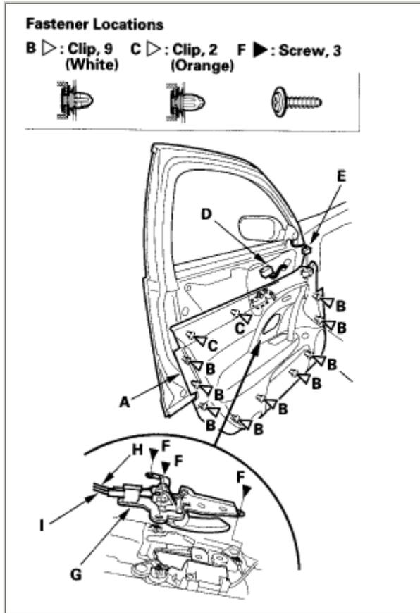
3. While holding the door panel away from the door, remove the screws (F), then remove the inner handle (G) from the door panel. **NOTE:** The inner handle cable (H) and the lock cable (I) are connected to the door panel. Do not pull the door panel up too far, or the inner handle cable will be damaged.
