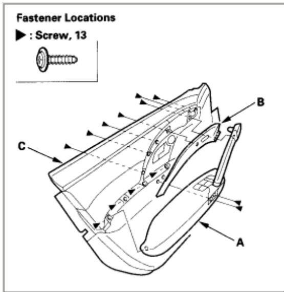
9. Remove the screws, then remove the grip/armrest (A) and the wood trim (B) from the door panel (C).
